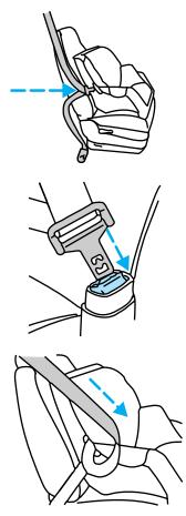
7. Pull the lap belt portion across the child seat toward the buckle and pull up on the shoulder belt while pushing down with your knee on the child seat.
